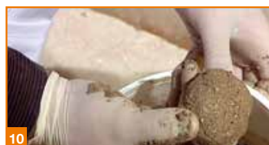
To check for appropriate malleability, the mortar should be moulded to a ball shape without falling apart.
